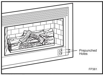
Fig. 11 Installing remote switch bracket.
